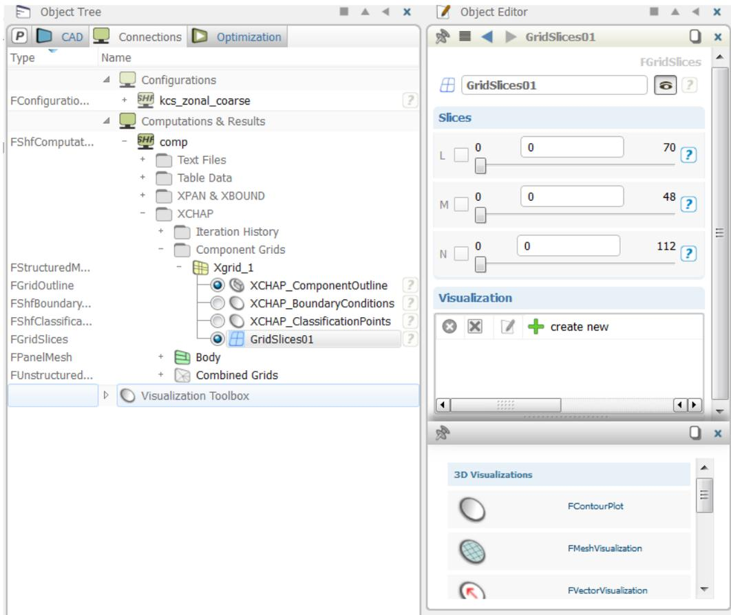
Grid planes in the three parametric directions L, M, N can be activated in the editor. The planes can be shifted in the corresponding parametric direction by moving the slider or entering the value. Try to change the location of the grid plane and zoom in to inspect the grid.
