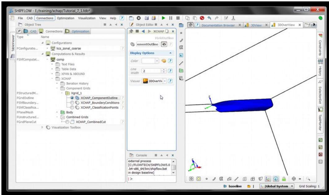
The GridSlice tool can be used for inspecting the grid planes in a 3d grid. The tool is created by selecting the Xgrid\_1 object and then selecting Create New in the empty row of the Visualization widget as shown in the picture below.
