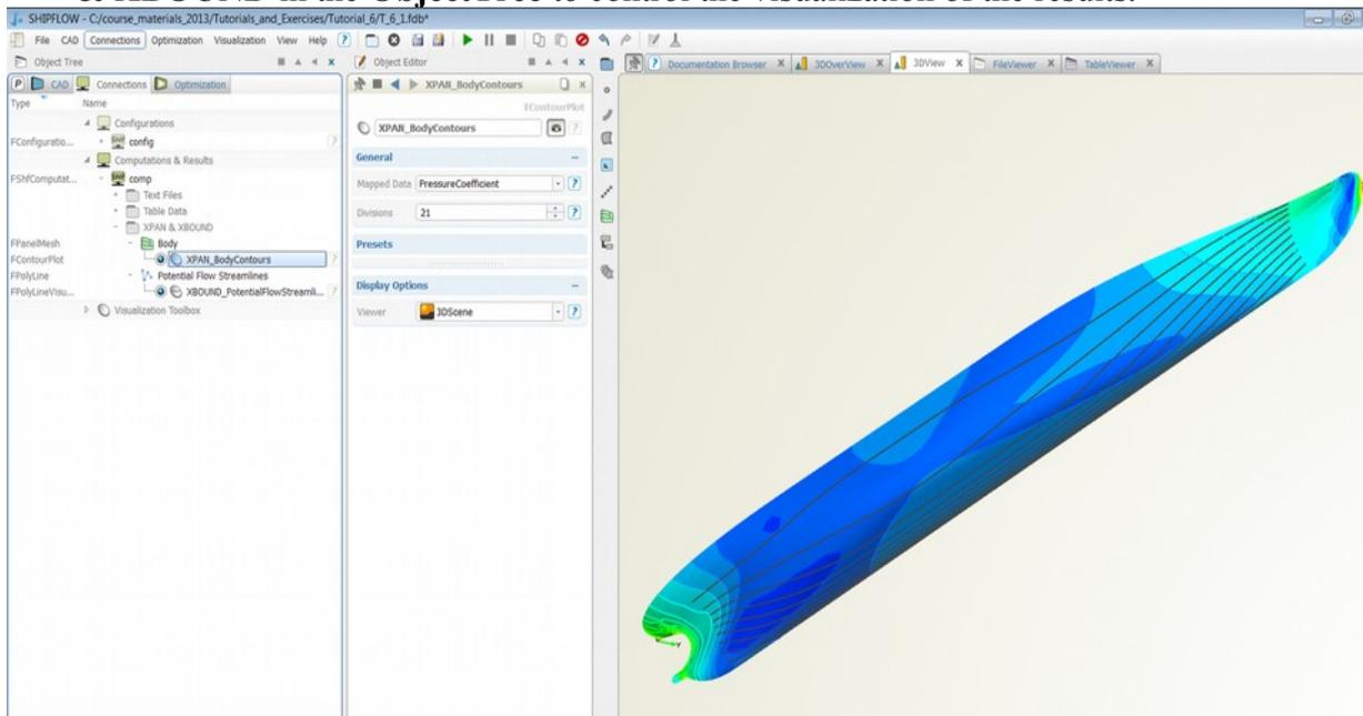
The next part of the tutorial will show some possibilities for the user to control the distribution of the potential flow streamlines. In our example we will try to get some additional streamlines on the side of the ship at midships. This can be done for example by specifying another value of the **ISTART** parameter that controls the location of points from which the streamlines are traced (up- and downstream).
