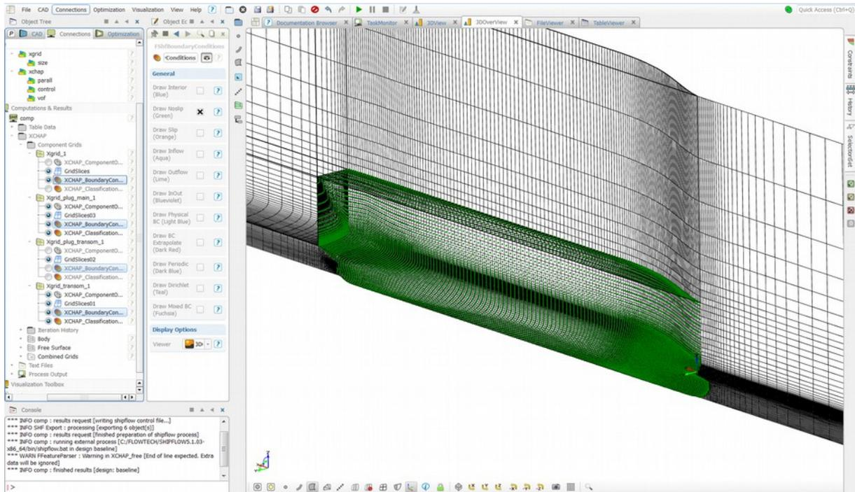
Looking on the surface mesh from a side one can see that there is a band of finer cells in vertical direction around the air-water interface. The number of cells in the girthwise direction can be set under the lower face of the refined region, in the refined region and above it using UETAMAX, AETAMAX, JMAXF and ETAMAX. The refinement dimension can be set using HUND and HABO to give non-dimensional distances from the still water plane in vertical direction.
