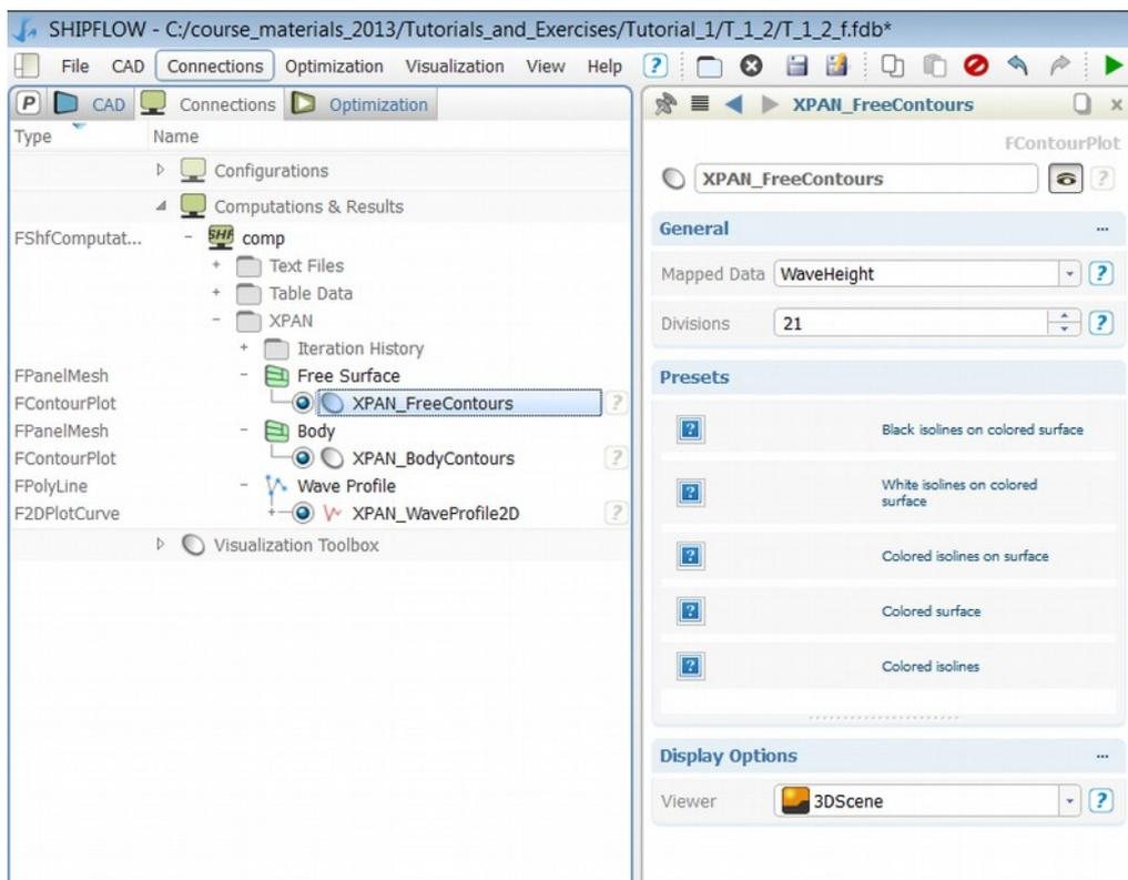
6. To change for example the wave pattern visualisation style go to **Object Tree | Connections | Computations & Results | comp | XPAN | Free Surface | XPAN** (or click on the free surface in the 3DView) and in the **Object Editor** change **Presets** to “Black isolines on coloured surface”. In a similar way the style can be changed on the hull panels
