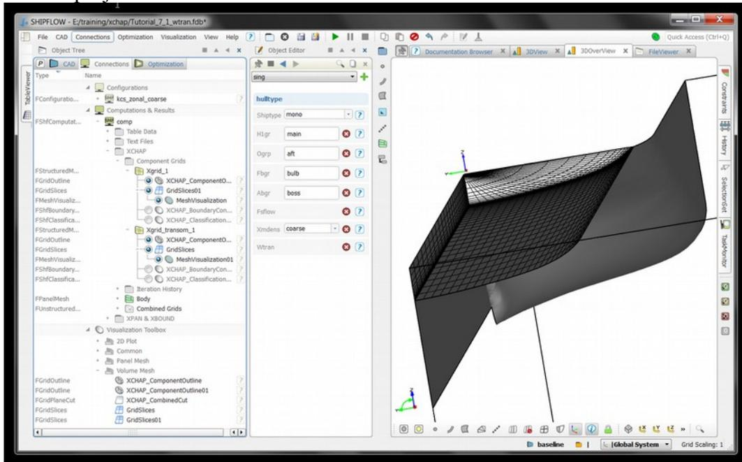
Note that two grids were created in XGRID, the Xgrid\_1 and the Xgrid\_transom\_1. You can see this under **XCHAP | Components Grids** in the Object tree. Two GridSlice tools have created in the picture above to visualize the grids.
