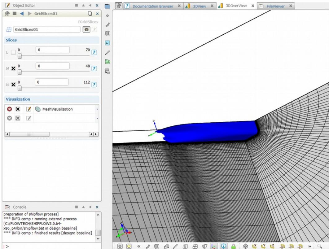
The boundary conditions can be visualized with the XCHAP\_BoundaryConditions tool which can be found in **XCHAP | Component Grids | Xgrid\_1** in this case. Activate the tool with the round button in the Object Tree. Press the text part to show the editor. Select for example the Noslip, Slip and Inflow boundary conditions. A coloured sphere is then displayed at the centre of each boundary cell face.
