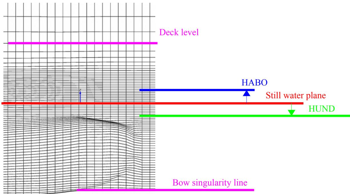
Now try to set the HABO and number of cells in girthwise direction to cover waves that are higher and keep similar cell size in the free-surface refinement band.
