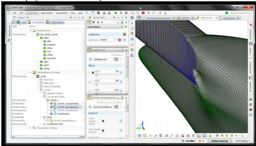
Use for example a GridSlice tool to display the surface grid and the folded surface. Show noslip and interior boundary conditions with the XCHAP\_BoundaryCondition tool.
