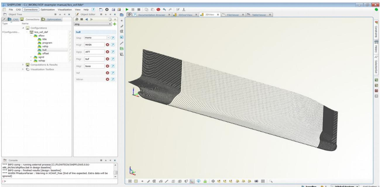
Run it for 0 iterations and display surface mesh on the hull and transom
